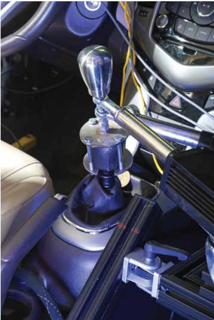
We expanded the test range of DEVCon, our electronic control system, by adding an auto-shift capability to evaluate vehicles with manual transmissions.
