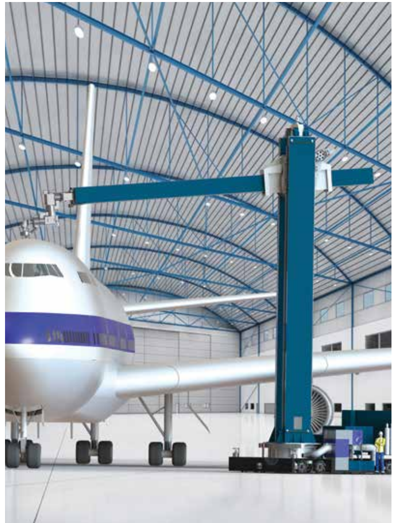
SwRI is developing the largest mobile robotics system in the world. The system combines a high-power laser with a mobile robotic platform and a laser scanner to efficiently and safely remove paint from aircraft and other large structures.
