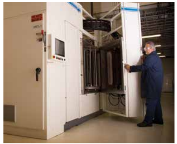
We acquired a large-format industrial coating system to complement our existing surface modification equipment. Using the SwRI-developed plasma enhanced magnetron sputtering process, engineers harden the surfaces of machine tools and other devices by applying specialized coatings.
