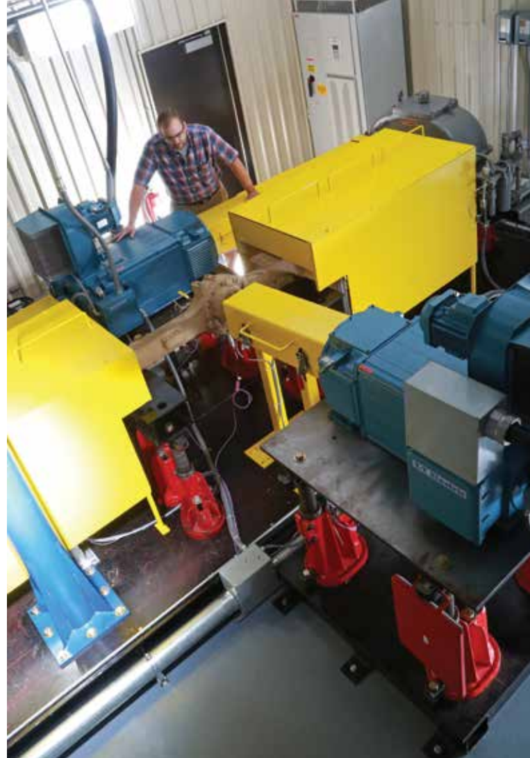
We developed a specialized axle test stand for evaluating gear oils used in military vehicles.
