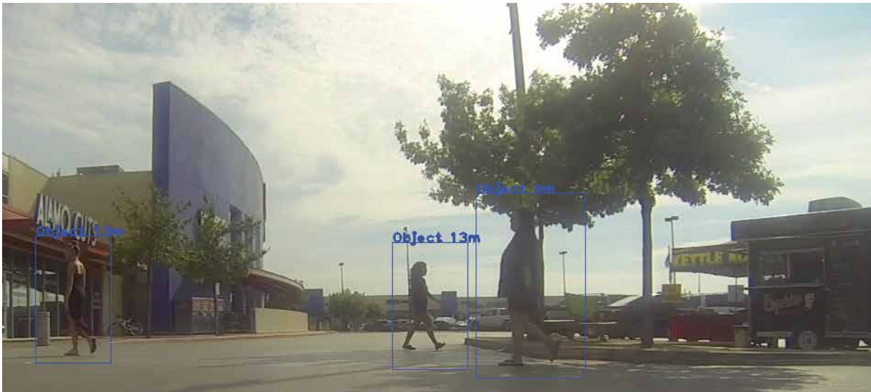
SwRI applied deep learning techniques and neural networks to help unmanned vehicles identify objects. Trained to identify pedestrians, cyclists, vehicles, traffic signs, and more, the system can detect objects of varying sizes at longer ranges.
