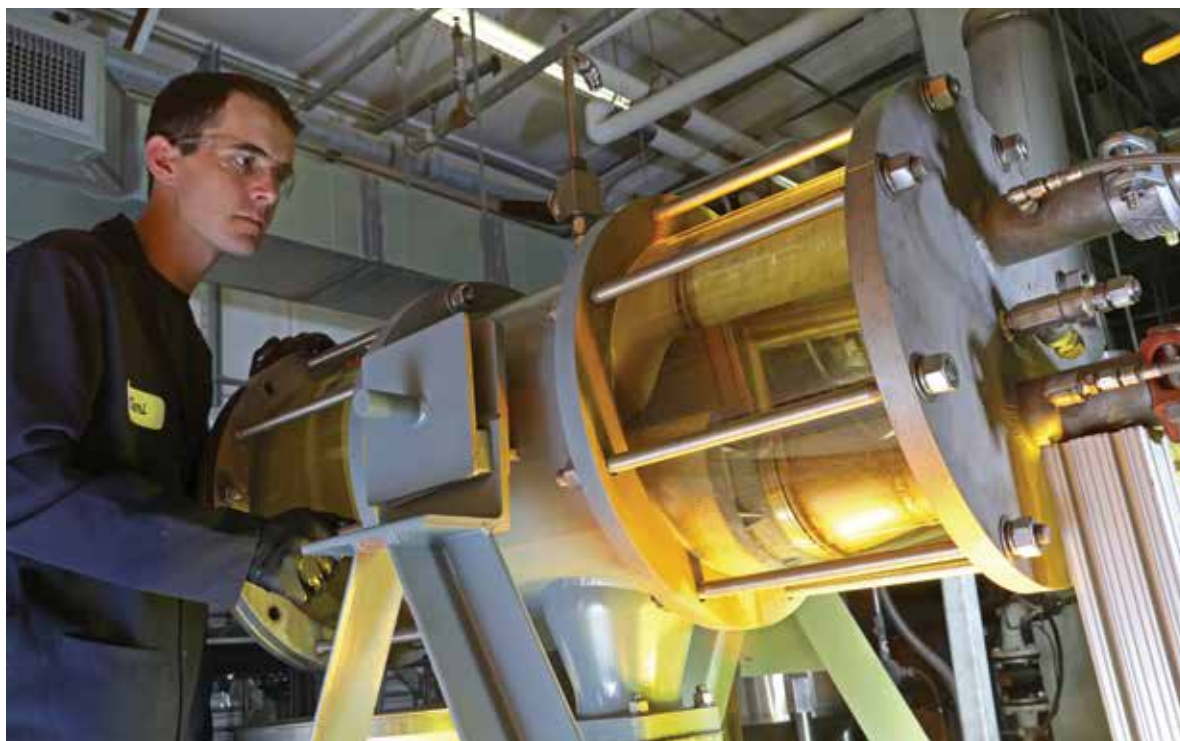
Our water mapping test rig evaluates how additives affect aviation fuels and how effectively filtration systems can remove water from the fuel.
