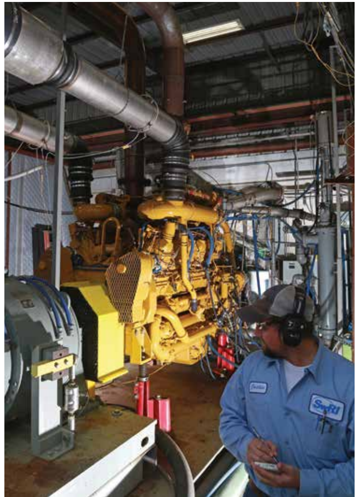
We designed this dual-fuel test stand to evaluate combining diesel fuel and natural gas in large, high-horsepower engines to reduce costs and lower emissions.
