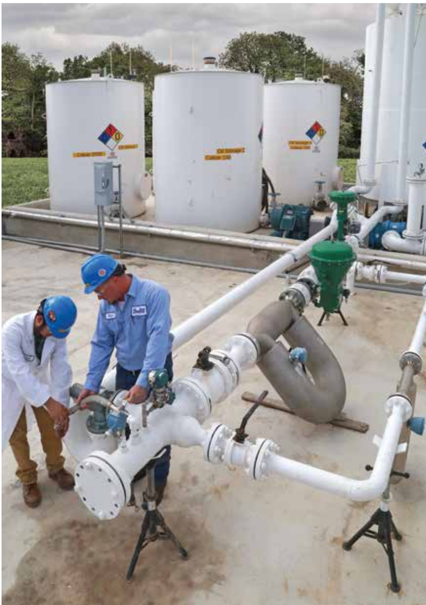
SwRI built this high-viscosity flow loop to test pumps, filtering elements, electrostatic separation systems, oil and water mixers, and other flow components under three-phase (oil, water, and gas) conditions.
