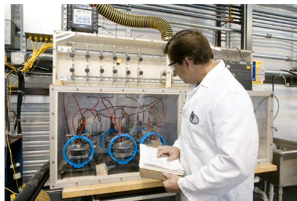
SwRI is investigating sulfide stress cracking resistance at different temperatures and under rigorous deoxygenation using a variety of test methods.
