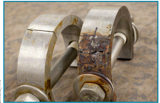
SwRI is currently undertaking a major joint industry program to evaluate stress corrosion cracking of materials in completion fluids for oil and gas production.
