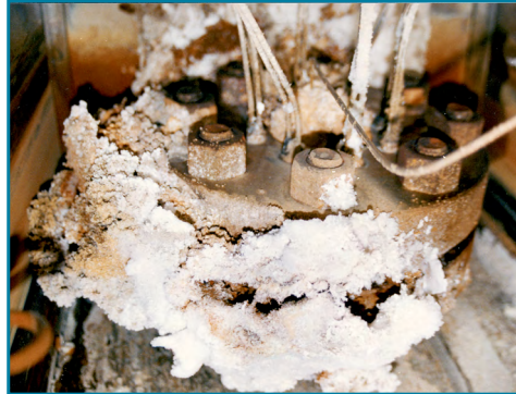
The effect of boric acid leakage from high-pressure, high-temperature fluids in flanged joints leads to deposits of borate and high corrosion rates. SwRI constructed facilities to simulate this process and conducted extensive testing.
