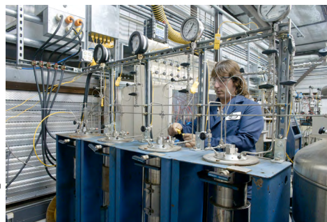
Advanced instrumentation is used for both standardized and unique specialized testing. SwRI conducts tests in the presence of high-pressure hazardous gases such as H 2 S with state-of-the-art analytical instruments.
