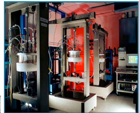
To measure service loads, SwRI-built stress corrosion cracking test frames can simulate a slowly oscillating load superimposed on a static load.
