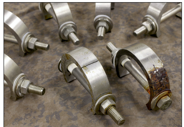
SwRI performed stress corrosion cracking (SCC) evaluations using C-rings. Specimens were exposed to a downhole simulated environment and evaluated for SCC.
