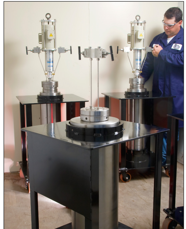
High pressure high temperature (HPHT) testing can be performed to determine stress cracking and/or mass loss corrosion effects under H 2 S, CO 2 , or other gaseous environments. Testing can be performed up to 650°F and 20,000 psi.
