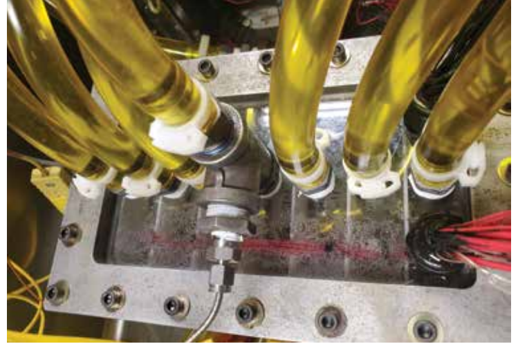
SwRI developed a flow rig to study the impact of direct immersion cooling on battery cell performance and aging.
