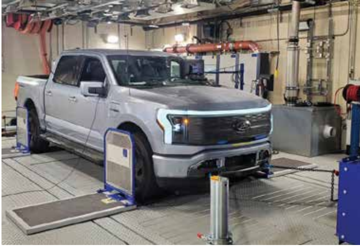
SwRI conducts range and efficiency testing on electric trucks using its all-wheel-drive chassis dynamometer.
