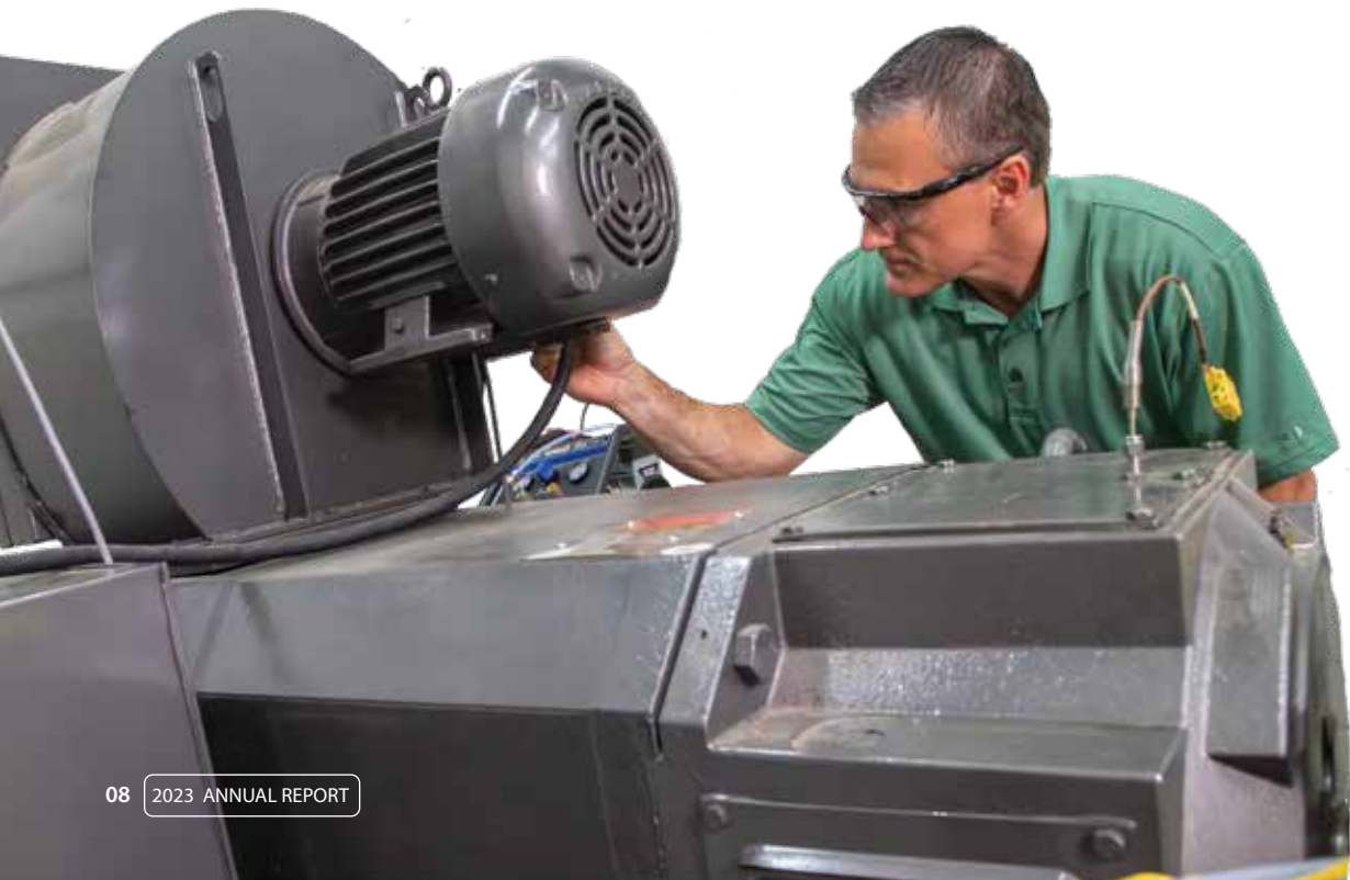
To support SwRI sustainability goals, engineers outfitted several test cells with regenerating drives to absorb engine power, converting up to 90% into electricity to offset power consumption or feed into the grid.
