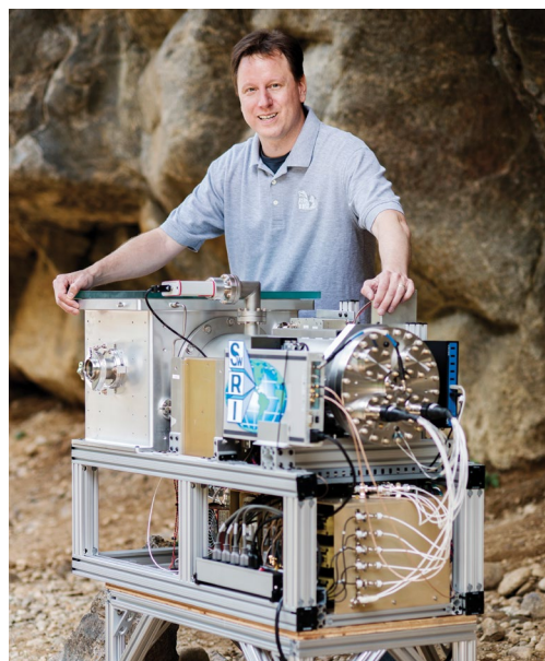
Dr. F. Scott Anderson displays a field prototype of the Chemistry, Organics, and Dating Experiment (CODEX) instrument.
