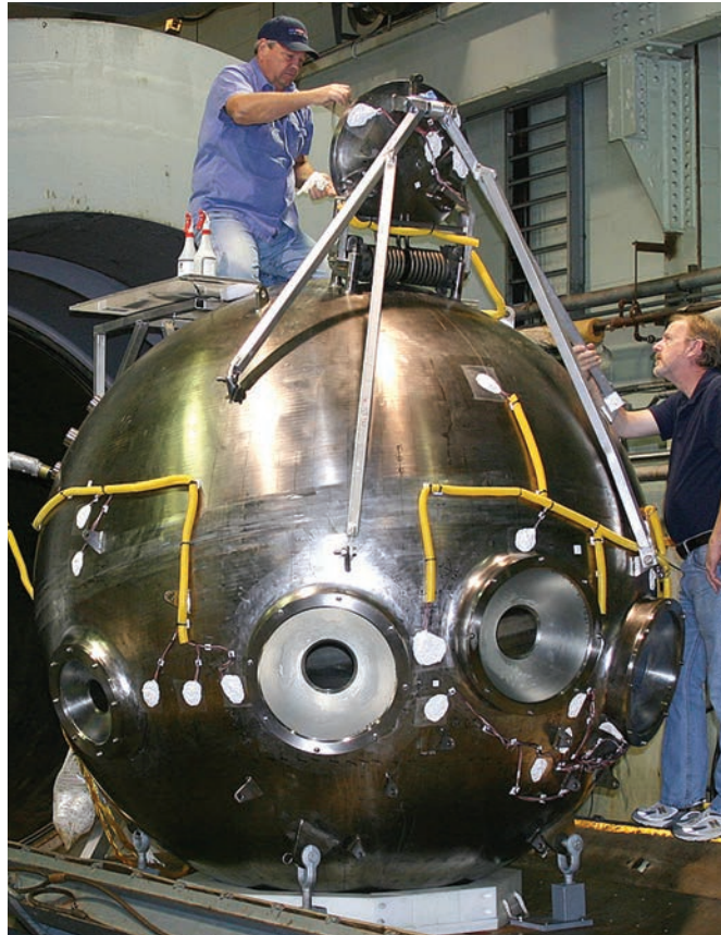
SwRI technicians install 80 strain gages in preparation for final hydrostatic pressure testing.
