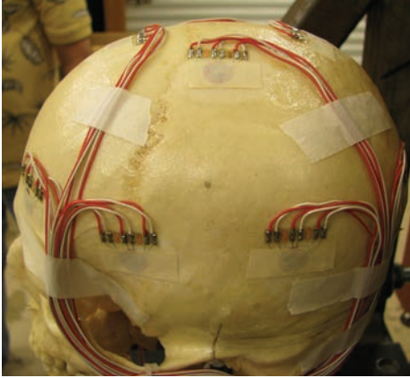
The human head surrogate has a suite of embedded instrumentation for measuring intracranial pressure, cranial strain and triaxial accelerations. The surrogate is supported by a 50-percent male neck assembly (right).
