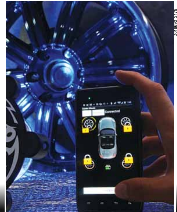
Aftermarket automotive wheels are a common target for thieves because existing locking devices (such as keyed lug nuts) are easily cracked. In 2012, SwRI helped a small business develop a better wheel security device: a wireless electromechanical combination wheel hub cover that locks and unlocks using a password-protected smart phone application.
