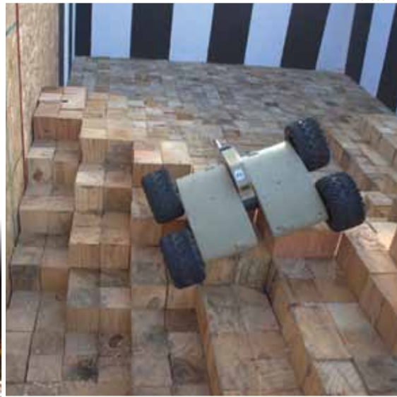
In a project for the National Institute of Standards and Technology, SwRI engineers helped design, build and run robot mobility test fixtures at Disaster City, a 52-acre facility in College Station, Texas, used to evaluate new robotic capabilities for use by emergency responders.
