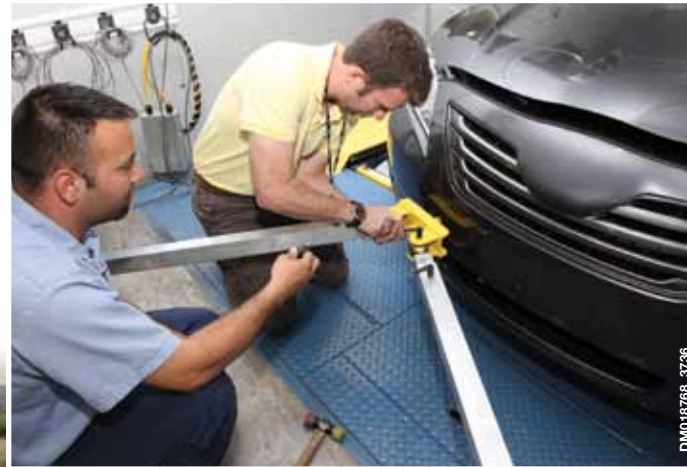
We upgraded our chassis dynamometer facilities with a rigid restraint system to improve the repeatability of fuel economy measurements, allowing us to help clients develop the next generation of fuels and lubricants.
