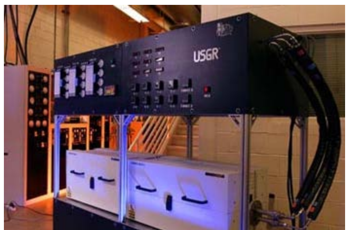
Figure 2: SwRI's Universal Synthetic Gas Reactor®
