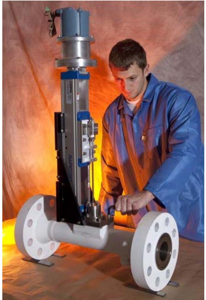
Figure 1. Iso-kinetic Sampling System for Measuring Liquid Entrainment at High Pressure.
