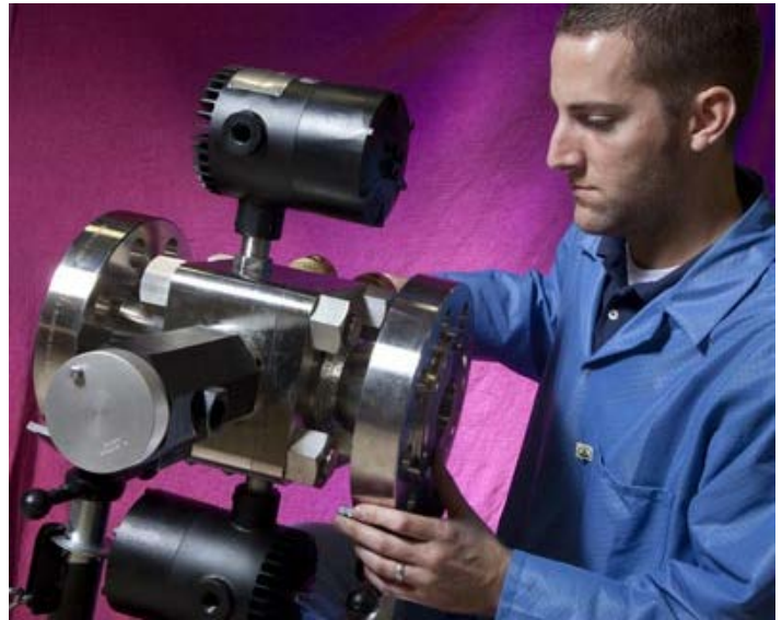
Figure 2. High-Pressure Multiphase Flow Visualization Device.
