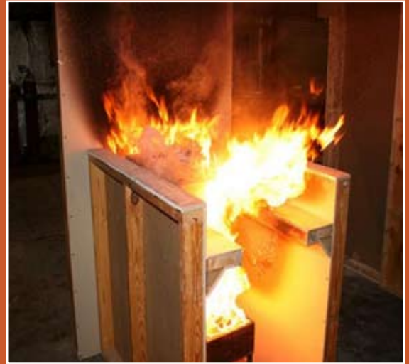
CA SFM 12-7A-4 Part A test for decking materials
