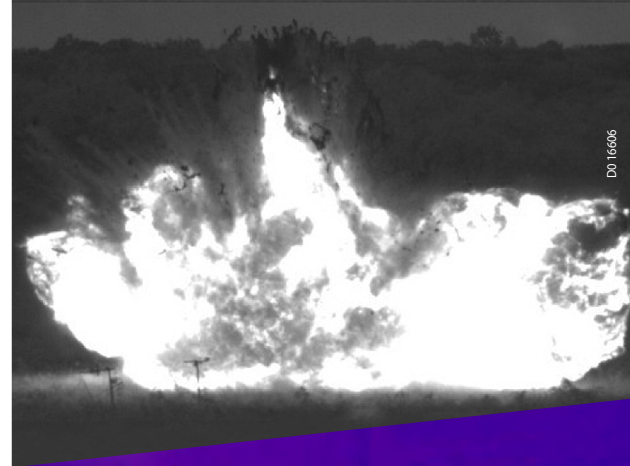
Infrared view of hydrogen ignition inside an engine compartment
