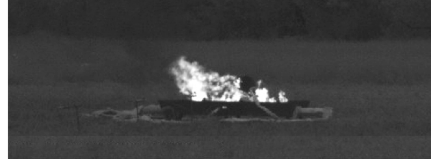
Catastrophic failure of a compressed hydrogen cylinder
