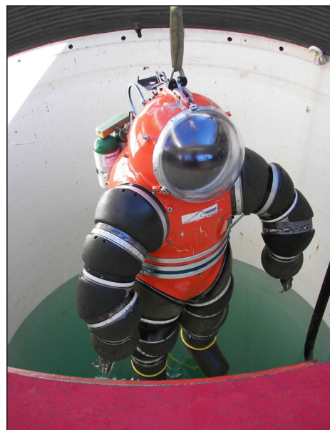
Diving suit subjected to hydrostatic pressure test
