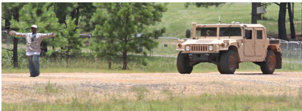
Gesture-based signaling instructs an unmanned ground vehicle during SwRI's demonstration of C4ISR applications.
