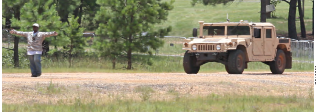
Gesture-based signaling instructs an unmanned ground vehicle during SwRI's demonstration of C4ISR applications.
