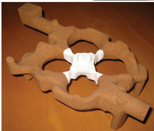
A traditional, reddish sand core contains white ceramic material at its center (left photo) to produce the finished product (right photo).
