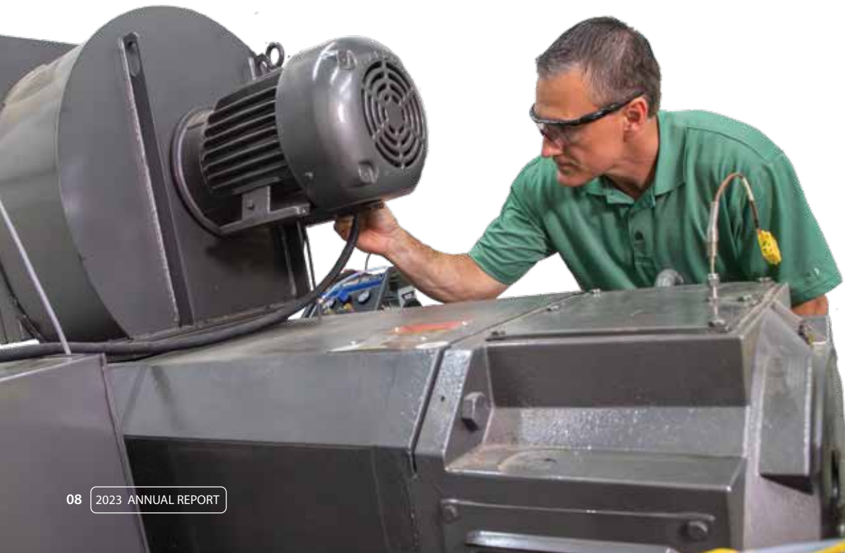
To support SwRI sustainability goals, engineers outfitted several test cells with regenerating drives to absorb engine power, converting up to 90% into electricity to offset power consumption or feed into the grid.
