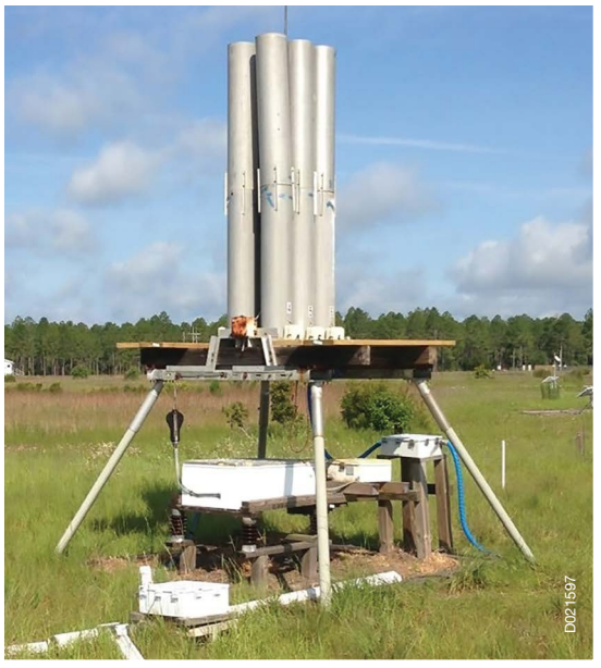
Scientists shot a wire-grounded model rocket from this launch pad into thunderclouds to trigger artificial lightning.
