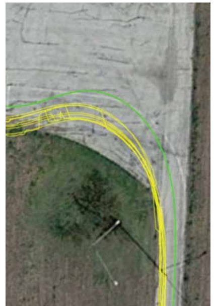
This image shows 10 automated vehicle loops around a slalom course. With Ranger, vehicle position (in green) varied by less than 5 centimeters, compared to GPS measurements (in yellow), which varied by as much as 2 meters. Ranger provides precise position and orientation measurements for automated vehicles using a ground-facing camera and localization algorithms.
