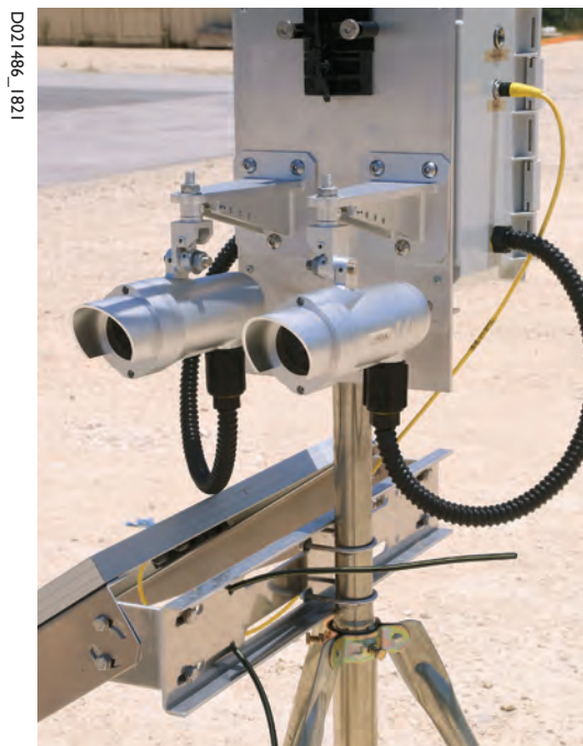
A "two-gun" laser system detects methane concentration of long distances. This sensor technology detects changes along the entire path as opposed to a stationary "point" sensor.
