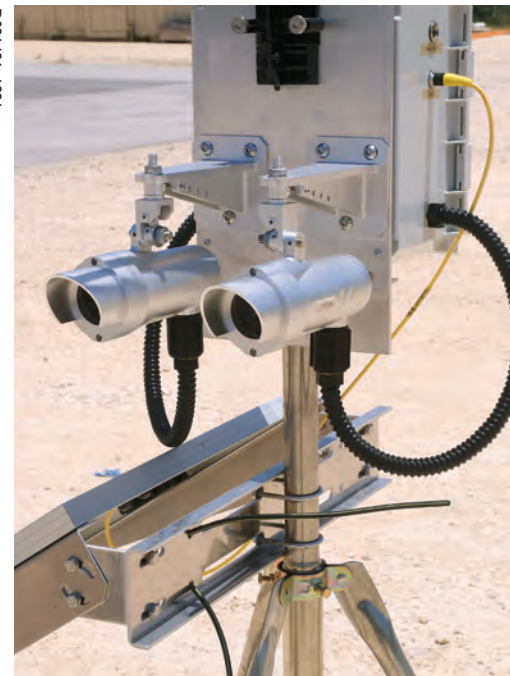
A "two-gun" laser system detects methane concentration of long distances. This sensor technology detects changes along the entire path as opposed to a stationary "point" sensor.
