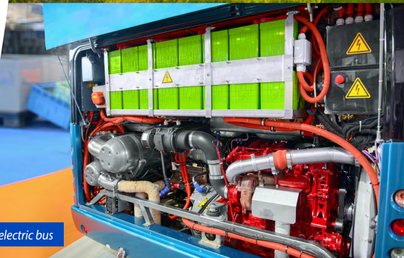
Ultra-capacitor-based start-stop mild hybrid
