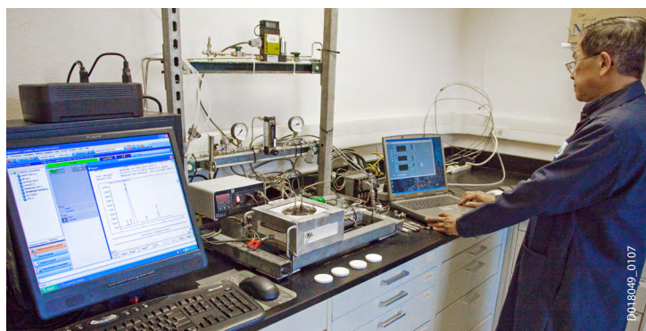
High-temperature CO 2 separation membrane evaluation system
