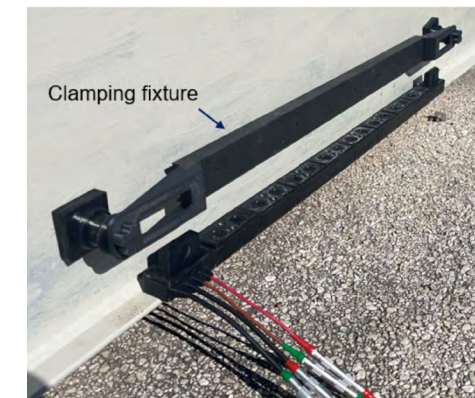
MsT probe with tank bottom extension
