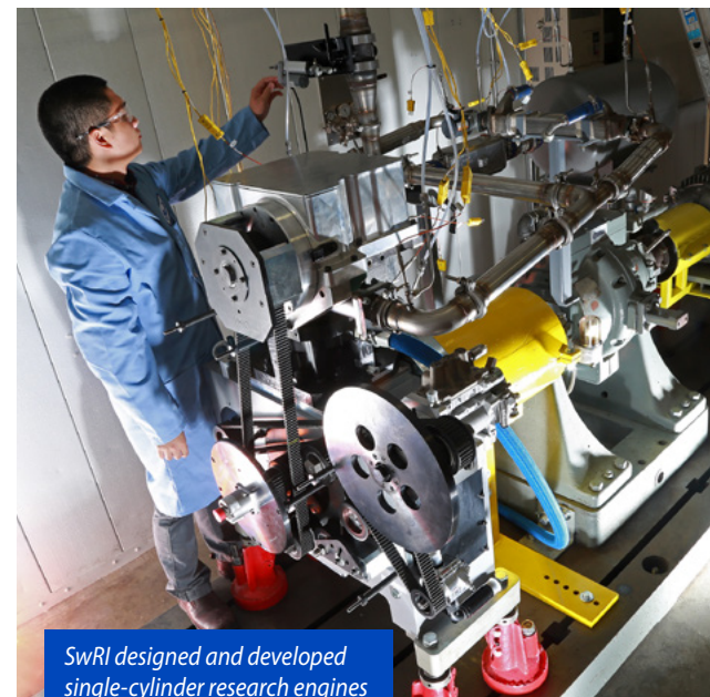
SwRI test cells include full transient dynos with dilute and raw emissions, high-speed crank angle synchronous data, and access to high voltage and power for additional accessories.
