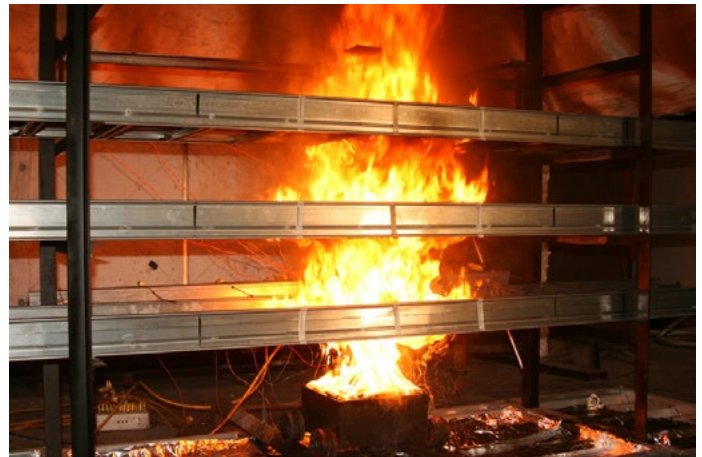
Full-scale test to evaluate fire propagation through a vertical stack of horizontal cable trays
