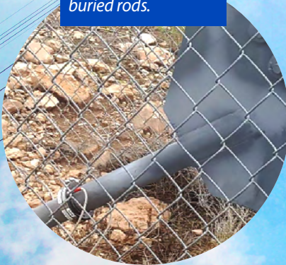
MsT probe for guided wave screening of buried rods.
