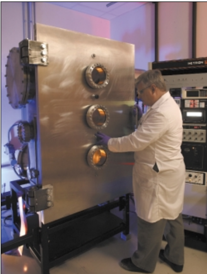
Engineers deposit optical coatings using a state-of-the-art cryopumped chamber housed in a dedicated Class 1000 clean room.
