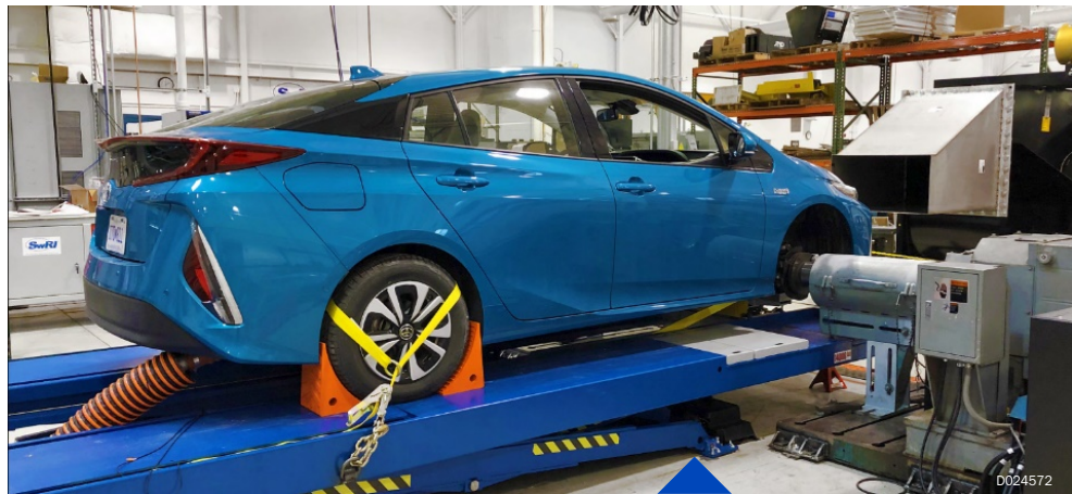
Vehicle positioned on dynamometer for testing
