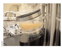
SwRI maintains a Shore Western six-station hip simulator used in conjunction with a radioactive tracer technology to measure minute amounts of wear in cross-linked UHMWPE and CoCr orthopedic materials.
