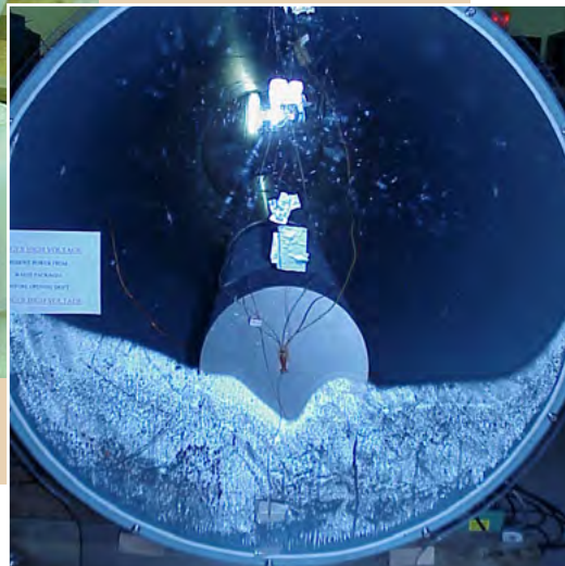
Two-phase flow experiments show zones of reduced temperature, elevated relative humidity and preferential condensation.
