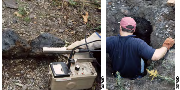
CNWRA scientists conducted field testing (left) to identify radiation hotspots for detailed sampling and characterization. Center scientists excavated a small abandoned slag pile (right) to collect fresh, unweathered samples for detailed laboratory analysis.
