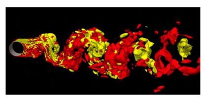
CNWRA performed three-dimensional simulations for high-speed flow over a circular cylinder to validate multiscale hybrid turbulence models.
