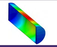
CNWRA engineers performed thermal analysis of spent fuel storage canisters to understand the temperature distribution pattern and maximum temperature locations during transportation.
