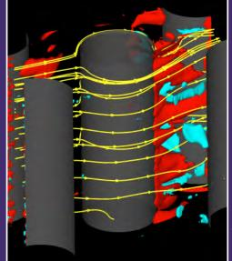
CNWRA engineers have simulated flow across staggered cylinders encountered in heat exchangers and reactors. The figure shows the streamlines and vorticity surfaces in the domain.
