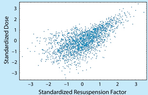
Scatterplot analysis of BDOSE output shows how variation in a sampled input parameter affects the calculated dose.
