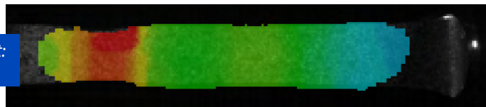
Split Hopkinson pressure bar (SHPB) test: DIC strain measurement (100,000 fps)
