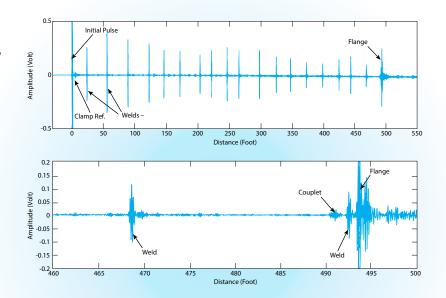
MsS data collected from a 16-inch diameter gas transmission line over a 500-foot-long section containing 19 welds and a flange connection (top waveform). The bottom waveform shows signals from a weld and couplet (type of piping branch) next to the flange.
