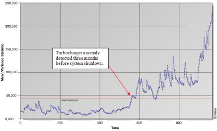
In this retrospective analysis, a turbocharger failure on a natural gas compressor had gone unnoticed by the system's fault codes, but nSPCT detected it automatically and three months prior to the system shutting down.
