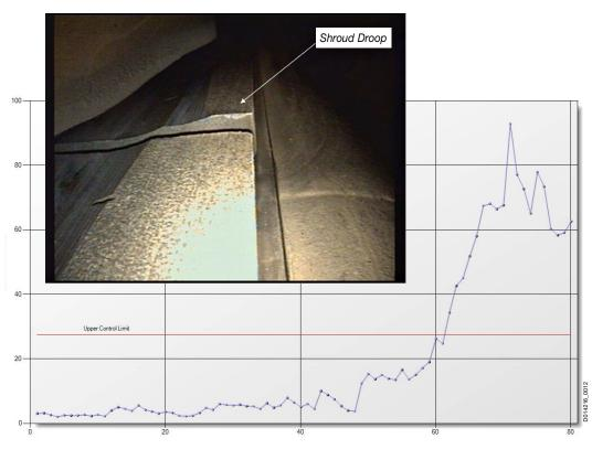
nSPCT algorithms detect and diagnose anomalous behavior in complex data sets. In this example, an F108 turbine shroud droop had gone unnoticed, but nSPCT detected it automatically and earlier than any other tools available to the Air Force.
