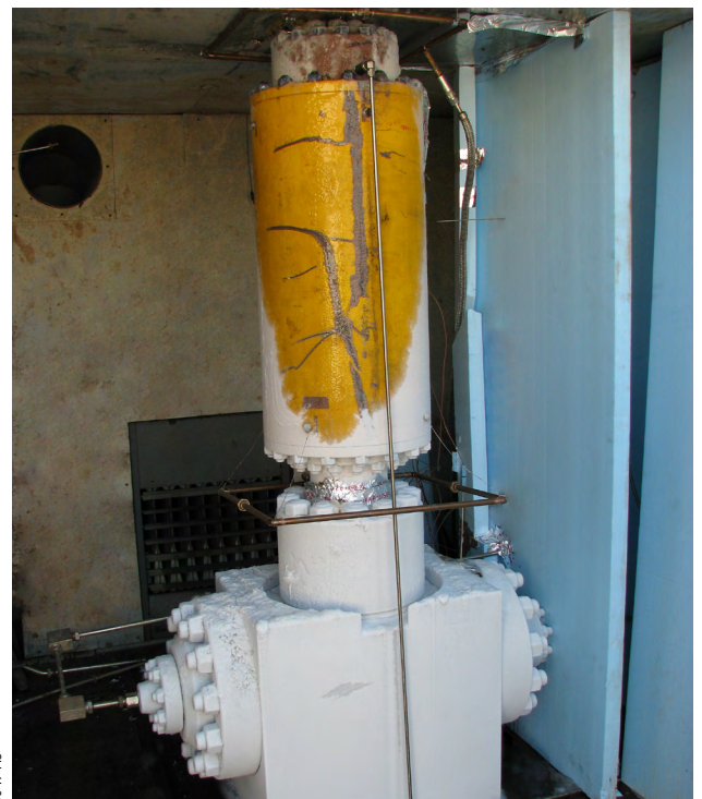
Valve and hydraulic actuator assembly undergoing low-temperature (-50°F) test
