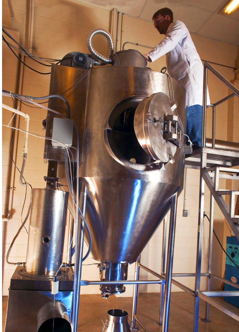
The SwRI production minor spray dryer can dry up to 25 kilograms per hour of water with rotary atomization or two-fluid atomization of the feed. Here a two-point collection (chamber and cyclone) system is installed.
