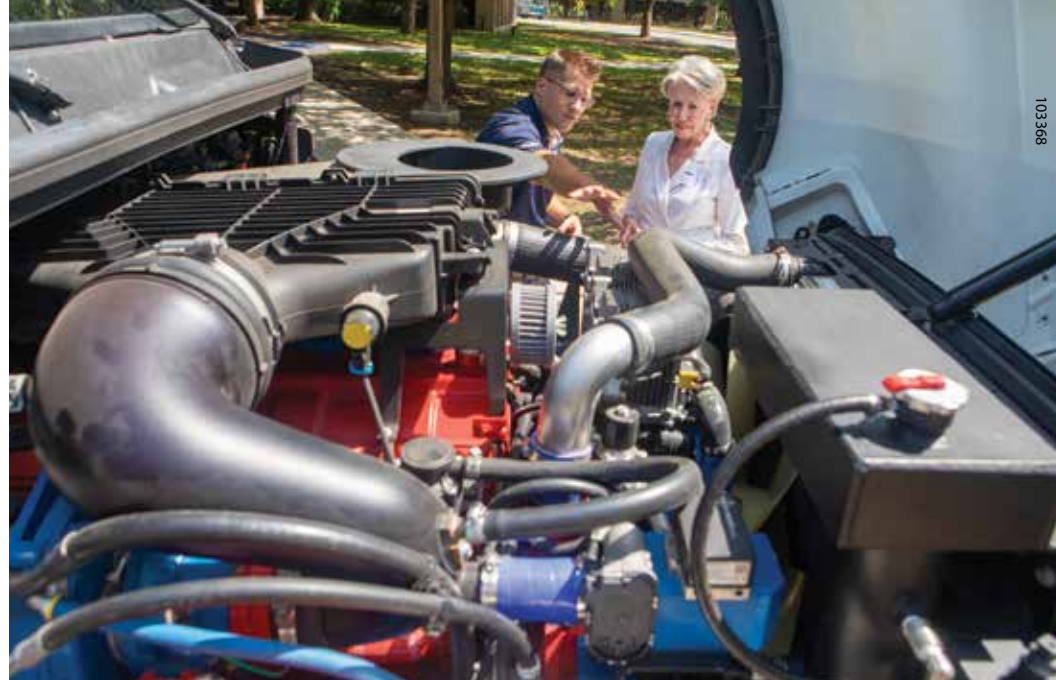
The H 2 -ICE engine in the demonstration vehicle used 90% of components from existing engines, leveraging existing supply chains and service networks to potentially bring these vehicles to market at scales able to affect decarbonization targets.
