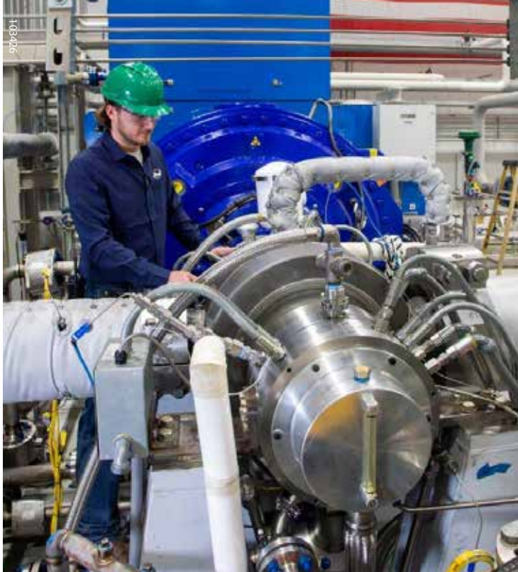
The Supercritical Transformational Electric Power (STEP) Demo pilot plant at SwRI generated electricity for the first time. The pilot plant's turbine achieved its full speed of 27,000 RPM, an operating temperature of 260 °C and generated a small amount of power.
