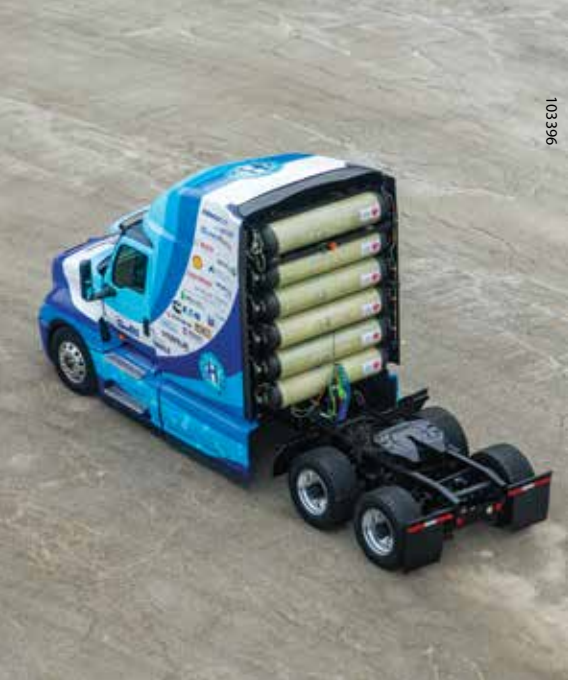
The transition to hydrogen fuel required a new fuel storage and distribution system. SwRI's demonstration vehicle also established how long-lasting diesel engines could be retrofitted to run on hydrogen.
