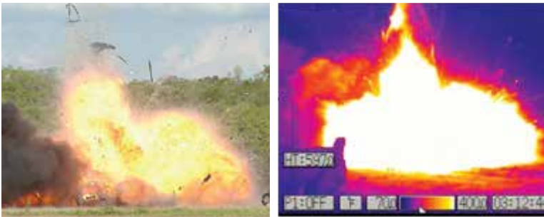
From a 1,600-acre remote location, SwRI evaluates compressed hydrogen cylinders installed in vehicles to understand the explosion hazards. Engineers collect data in the infrared to characterize catastrophic failures.
