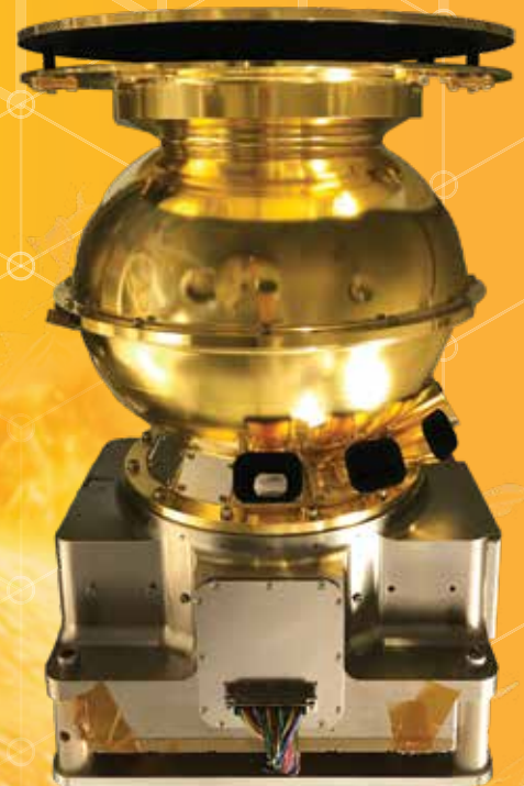
CoDICE combines the capabilities of multiple instruments into one patented sensor about the size of a 5-gallon paint bucket and weighing about 22 pounds.
