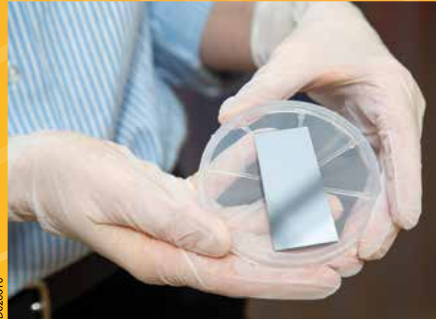
SwRI space scientists collaborated with materials specialists to create more effective particle detection surfaces for spacecraft instruments. Pictured is a conversion surface substrate developed specifically for the IMAP-Lo instrument.
