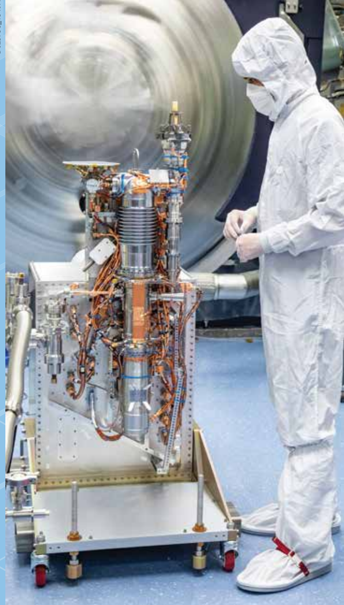
Space scientists used IR&D and NASA funding to develop MASPEX, a groundbreaking new mass spectrometer for the Europa Clipper mission to study the potential habitability of Jupiter's moon Europa.
