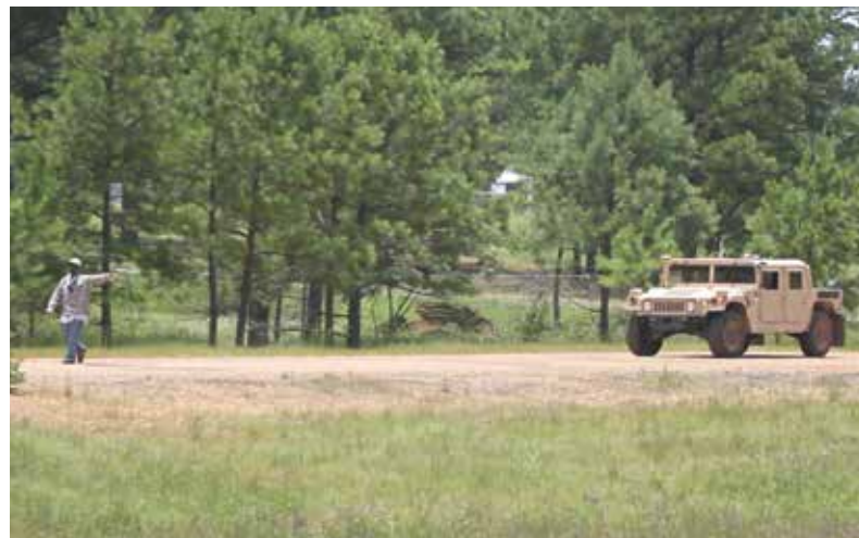
SwRI developed gesture recognition capabilities for automated driving systems used in military, highway work convoy and other applications. Image-processing algorithms identify and distinguish different arm gestures from a designated pedestrian that allow more natural, efficient interaction with an automated system.
