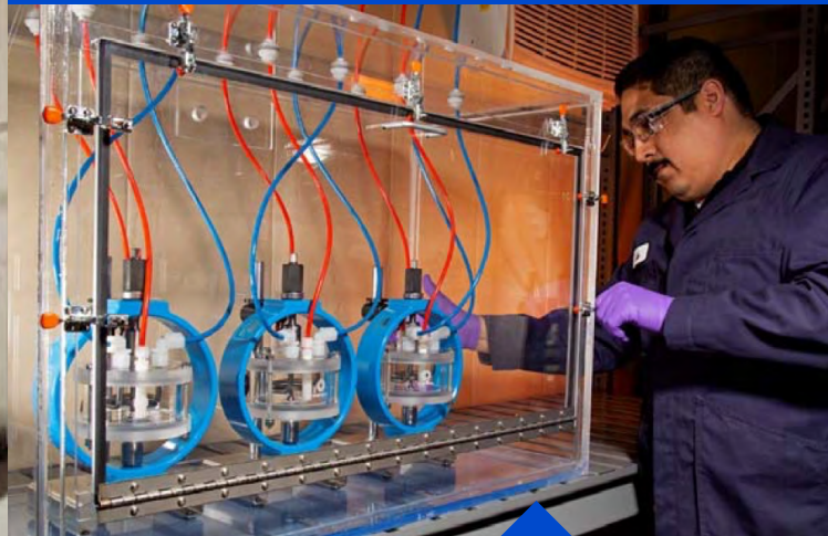
An SwRI technician prepares environmental test cells to simulate corrosion attack under service conditions.
