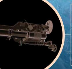
The novel MASPEX instrument provides **50** times finer resolution than other space spectrometers. At 3 feet long, it provides a 4,800-foot flight path as ions bounce **800** times back and forth to reveal chemistry.
