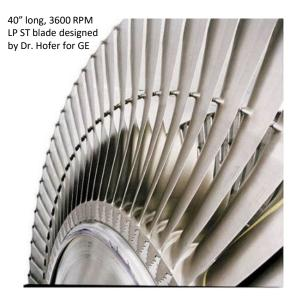
LP Steam Turbines have homogeneous condensation of up to 12% liquid
