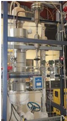
Patented high pressure circulating fluidized bed reactor
