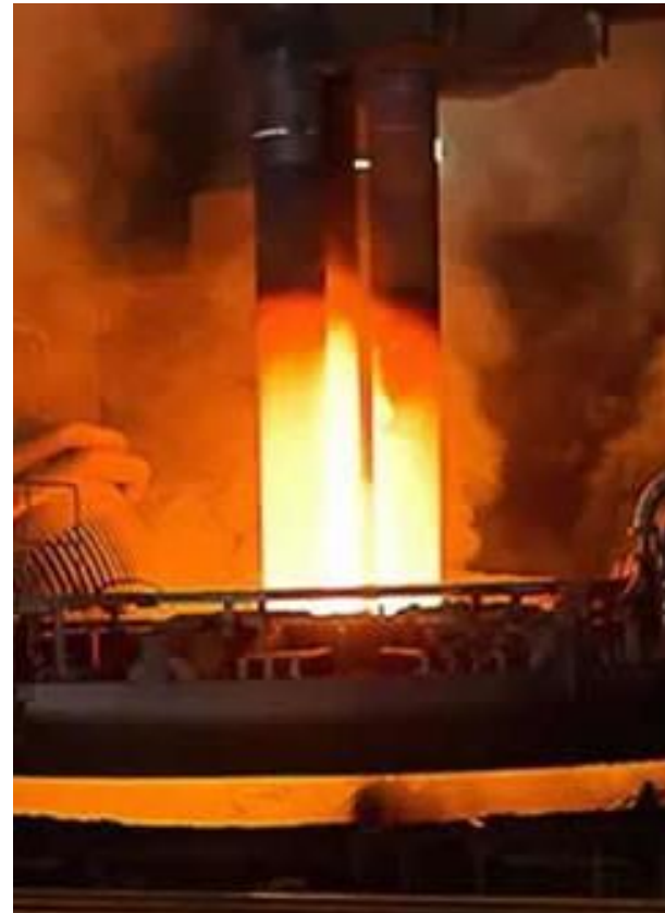
3 graphite electrodes being lowered into an AC electric arc furnace to strike an arc and make steel.
