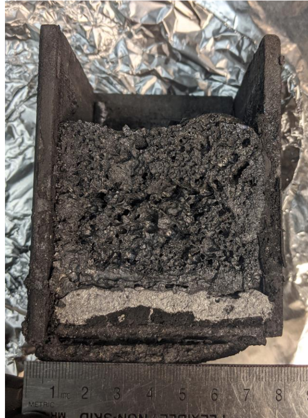
Metallic iron (bottom) reduced electrolytically from a molten sulfide slag (top)
